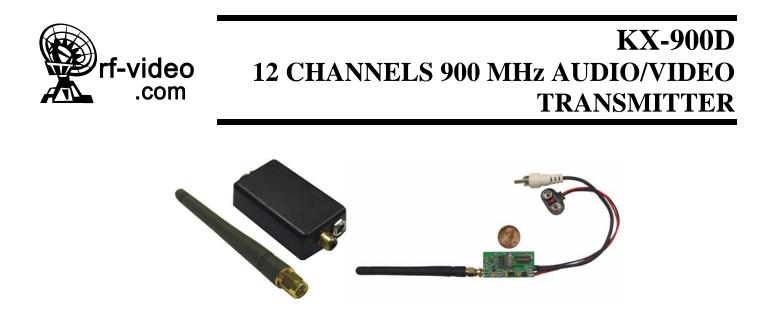
This small video transmitter for UHF is an excellent solution for video surveillance or experiments. The transmitter KX-900D is a 12 channels unit. It has 80 mW RF power. Dimensions: 2.4" X 1.5 "X 0.7". This transmitter sends a perfect color or B&W image to 900 MHz receiver including sound portion as well. Recommended receiver is M-808.
