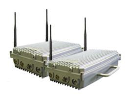
XLSW-5800 is excellent low cost microwave link for 5.8 GHz. It comes with 600 mW transmitters with 8 channels, (two transmitters are built-in); 8 channels receivers, (two receivers are built-in), 4 Omni directional antennas AX-58R; Capacity: 2 Video / 4 audio channels, the receiver has built-in low noise amplifier for increased sensitivity and bandpass filters. Operating frequency: synthesized. This link is Professional and it is
